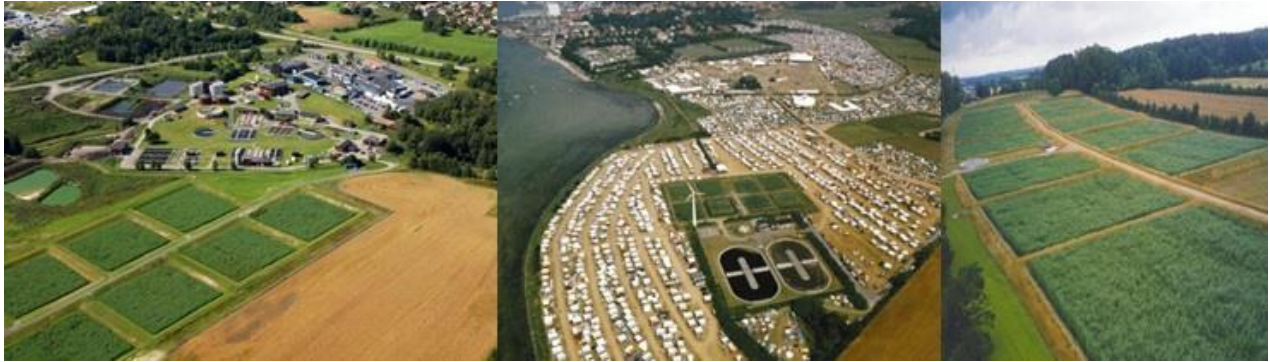
Figure 2: Example of excellent performances of sludge treatment reed beds – Skövde (2003, 1.200 tonnes of dry solids per year; left), Rudkøbing (1992, 250 tonnes of dry solids per year; middle), Kolding (1998, 2.000 tonnes of dry solids per year; right) 5
