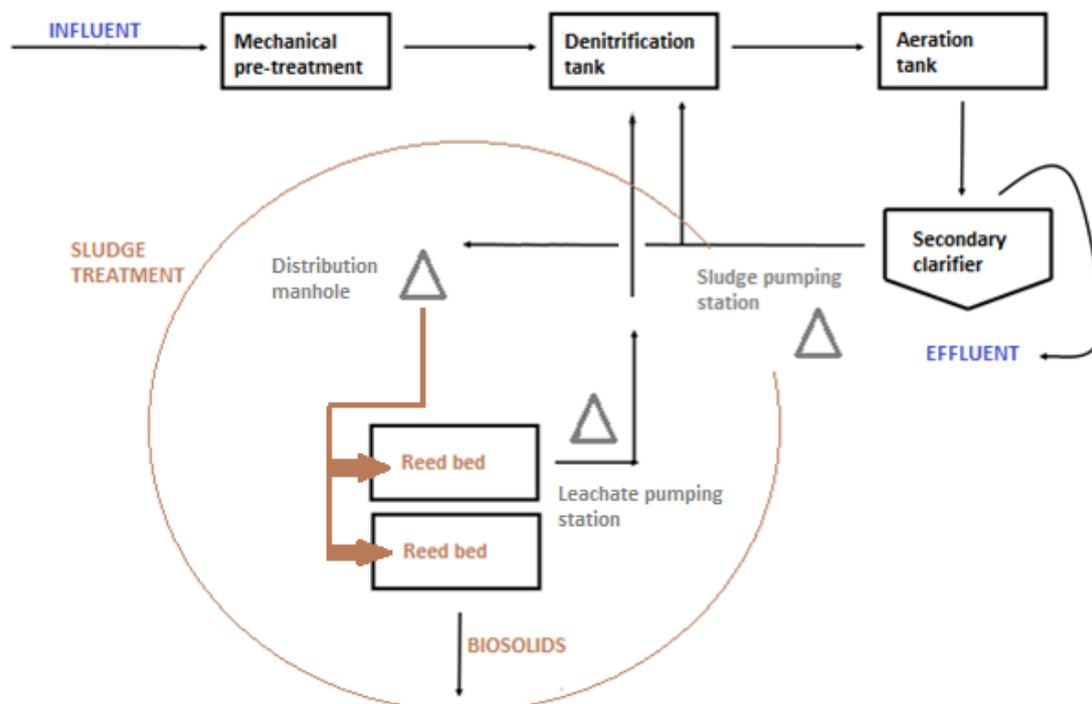
Figure 9: Flowchart diagram of operating sludge treatment in Mojkovac
