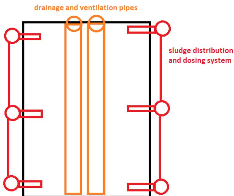
Figure 26: Sludge dosing system (red) and leachate collection system (orange)
