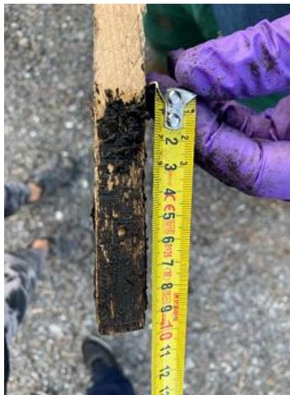
Figure 19: Sludge height in RBs Mojkovac.
