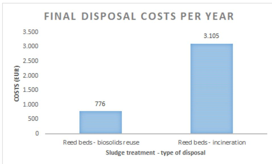
Figure 41: Final disposal costs taking into the account filling cycle of 20 years (forecasted sludge production).
