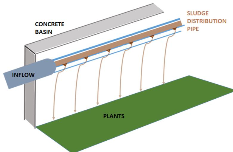
Figure 8: Sludge distribution pipe
