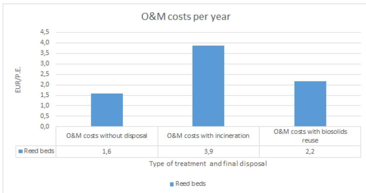
Figure 42: O&M costs for sludge treatment per year
