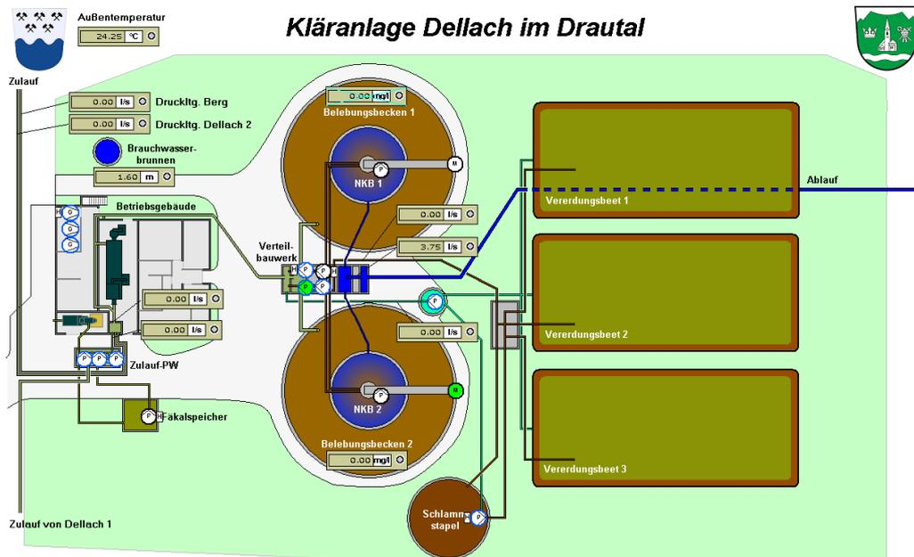
Figure 25: WWTP Dellach process scheme<sup>27</sup>
