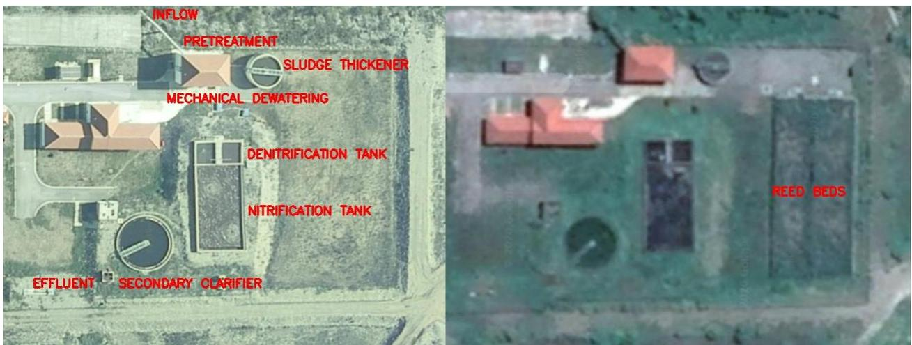
Figure 6: Aerial shot of WWTP Mojkovac before (left) and after RBs installation (right)<sup>16</sup>
