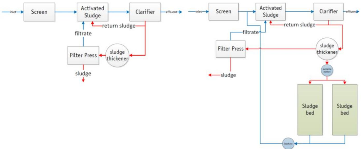
Figure 7: The process flowchart of WWTP Mojkovac with mechanical dewatering (left) and natural dewatering (right)<sup>17\*</sup>
