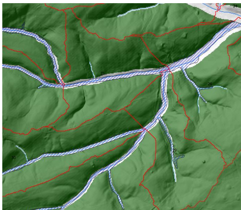
Figure 9. Example of the landscape unit creation technique creating a buffer 10x the width of the channel (white). The pre-determined approximate wetland restoration project areas (blue hatched lines) have been included for reference.
