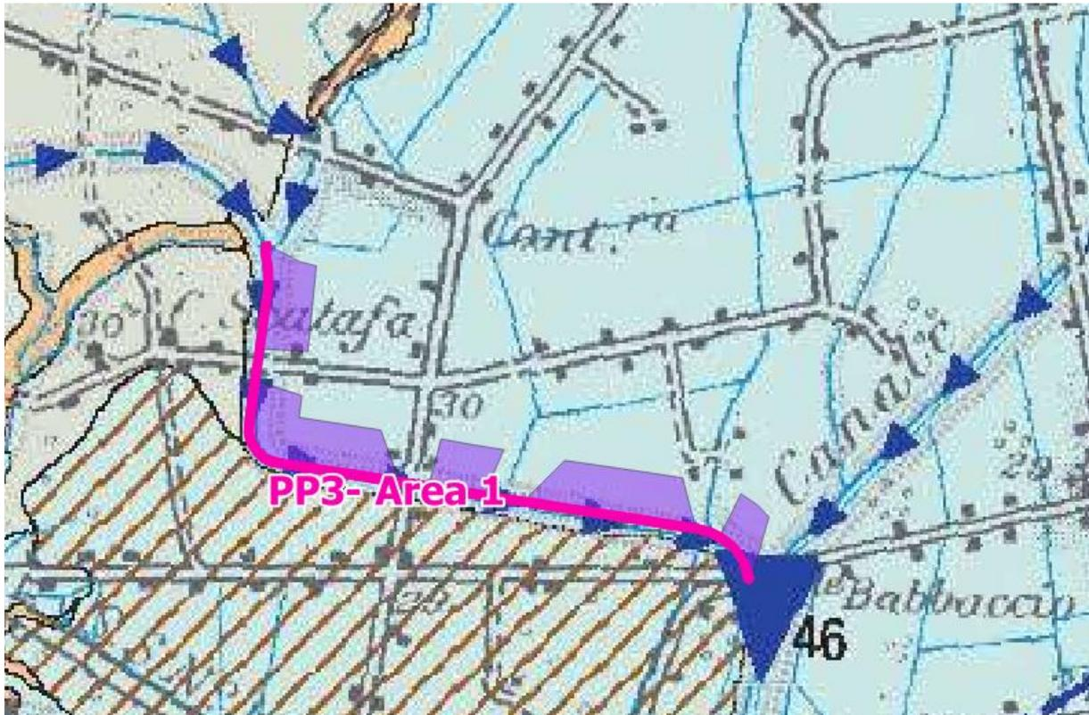
**Figure 33.** Close-up of the sub-basin map with the area drained to the buffer strip
