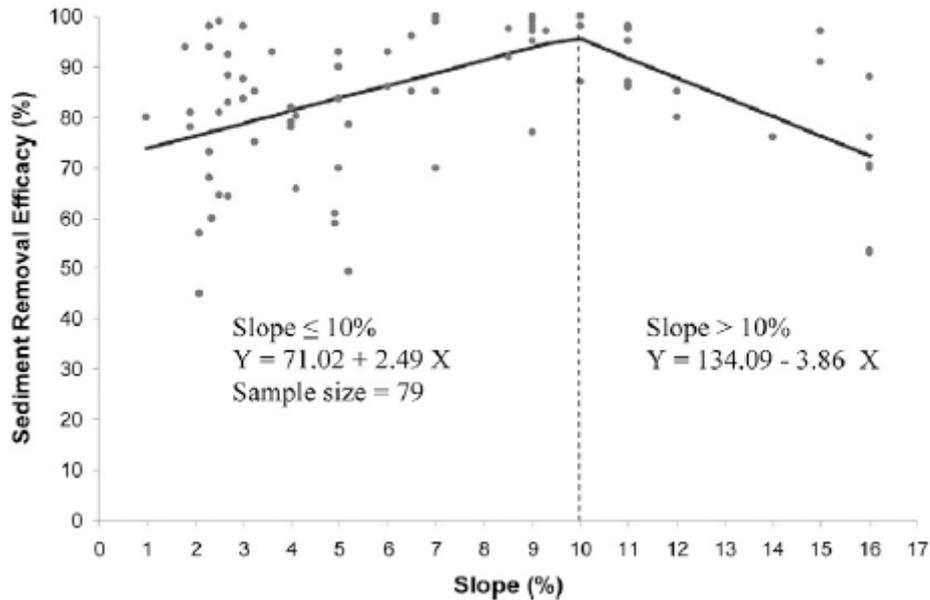
**Figure 22.** Correlation between sediment removal efficacy and buffer slope (Zhang et al., 2010)
