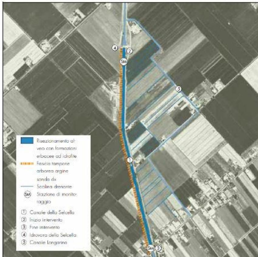
**Figure 17.** Buffer Strip and self-purification enhancement of the Selcella Canal
