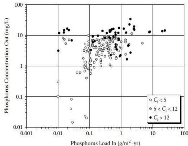
**Figure 21.** Outlet TP concentration versus TP loading for HF from Kadlec and Wallace (2009); data from 193 HF wetlands
