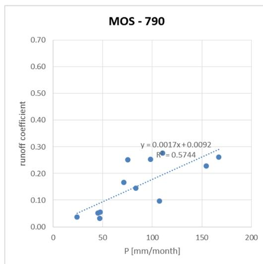
**Figure 49.** Linear fitting of the runoff coefficient equation for the sub-basins of interest
