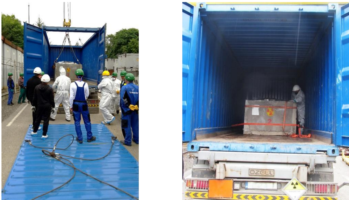
Figure 19. The load being placed (left) and secured (right) in a 20-foot ISO container
