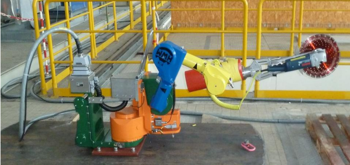
Power Manipulator attached to “OilQuick” coupler with grinder and 350 mm disc.
