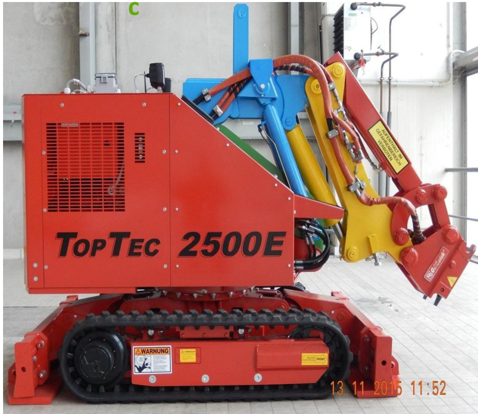
Remote operated demolition vehicle with remote rescue equipment
