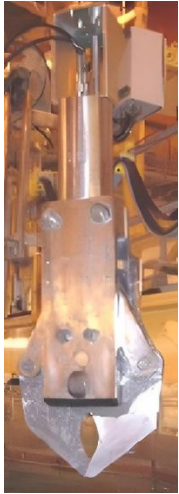
Figure 19: On the left, a hydraulic cutting shear used in the dismantling of the Chooz A nuclear power plant (France); on the right, the hydraulic cutting device used for the segmentation of control rods at the Ågesta nuclear power plant (Sweden) [4]
