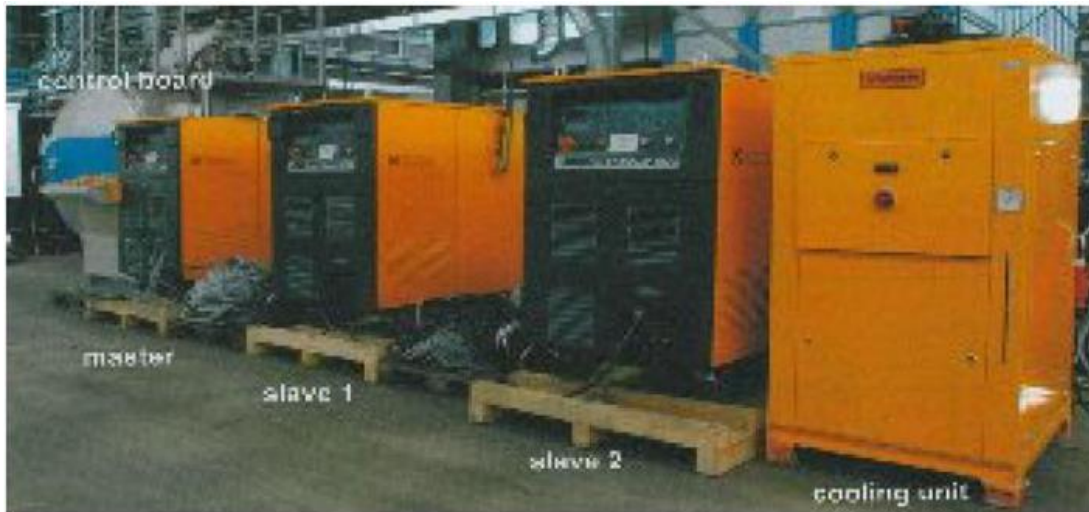
Figure 8: Plasma power sources with control board cooling unit and supply lines [2]
