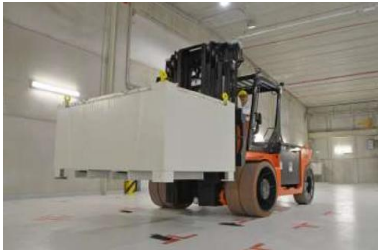
Figure 21. Test handling of a CP-5.2 container using an electric fork-lift
