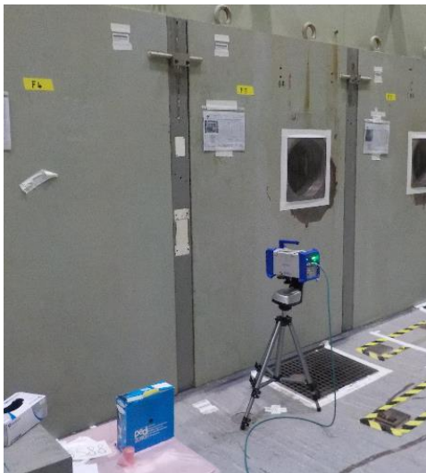
A. Background measurement in front of the hot-cell G (the hot-cell was closed with the lead door)
