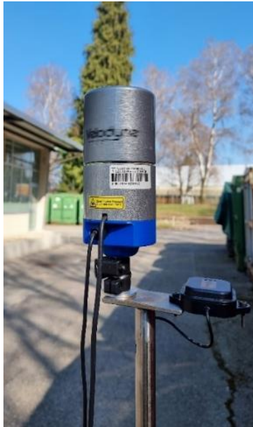
Velodyne LiDAR scanner (grey cylinder) and ANN-MB antenna for GNSS (flat black patch)
