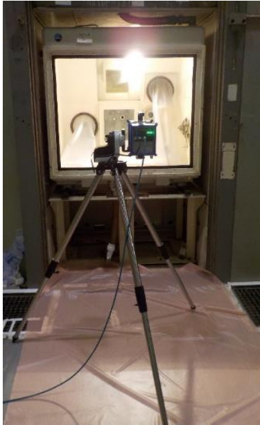
A. Background measurement in front of the hot-cell G (the hot-cell was closed with the lead door)
