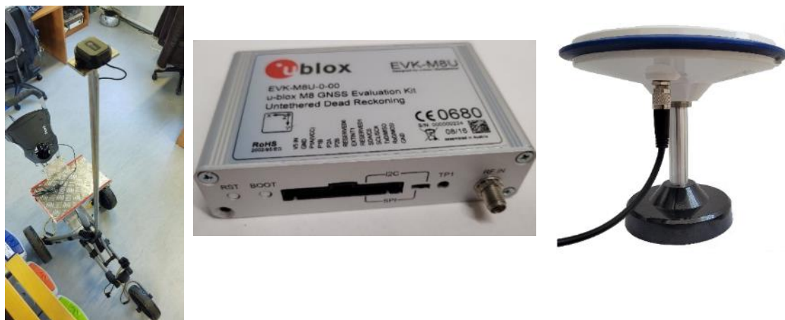
a. Extend antenna position b. The EVK-M8U evaluation board integrating the U-blox M8U receive c. Beitian BT-200 antenna
