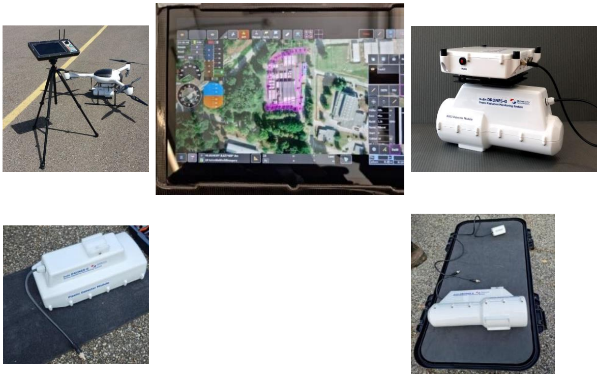
Figure 11: (Top) The UAS, the flight planner software and the radiological device DRONES-G NAI3 (source contractor). (Bottom) Plastic scintillator and the NaI 3x3" nuclear detector.
