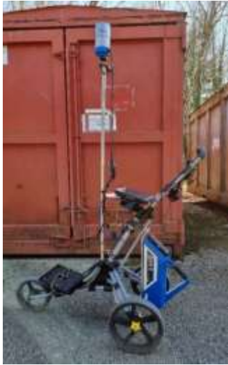
Figure 34: Mobile Laser Scanning Platform coupled with a gamma detector (NaI radiological identifier detector)
