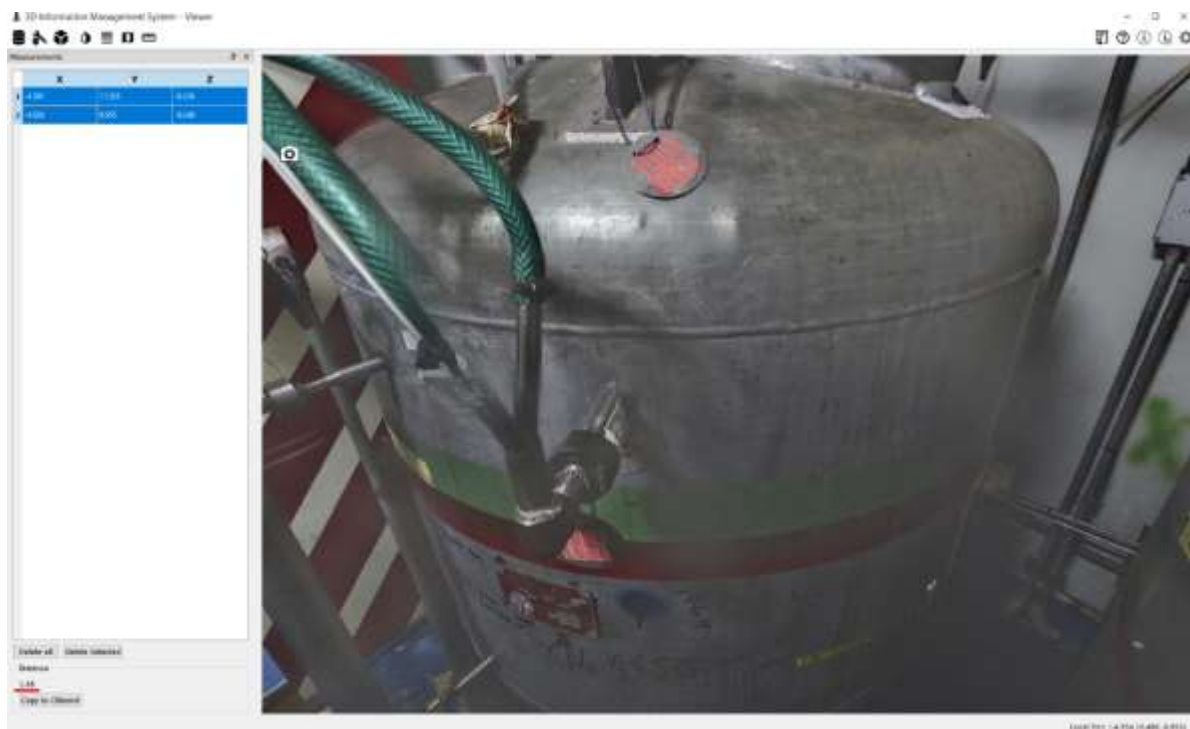
Figure 25: Result of the tank diameter measurement: 1.48 m visible in the bottom of the Measurement pane (where a red line was added to the screenshot)
