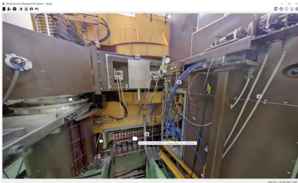
Figure 29: 3DIMS view of Cyclotron where component tags are visible: pointed heptagons; hovering a mouse above the tag shows its name – in this case C00163001LB0010
