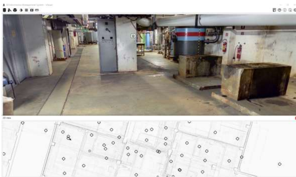
Figure 13: Example of the confusion created by “transparency” of 2D maps (source 3DIMS software)
