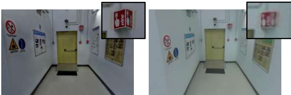
Figure 4: Part of spherical image with zoomed in detail (Left: Static scanner, Right: MLSP)
