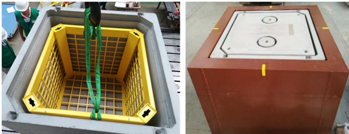
Figure 12: Inner steel basket & external steel shielding
