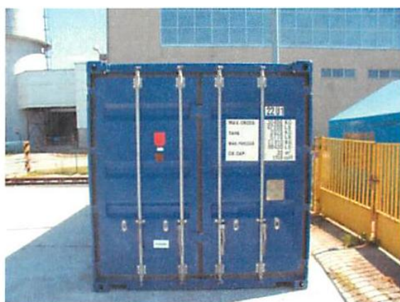
Figure 14: ISO 20' container for transport of RAW in Slovakia
