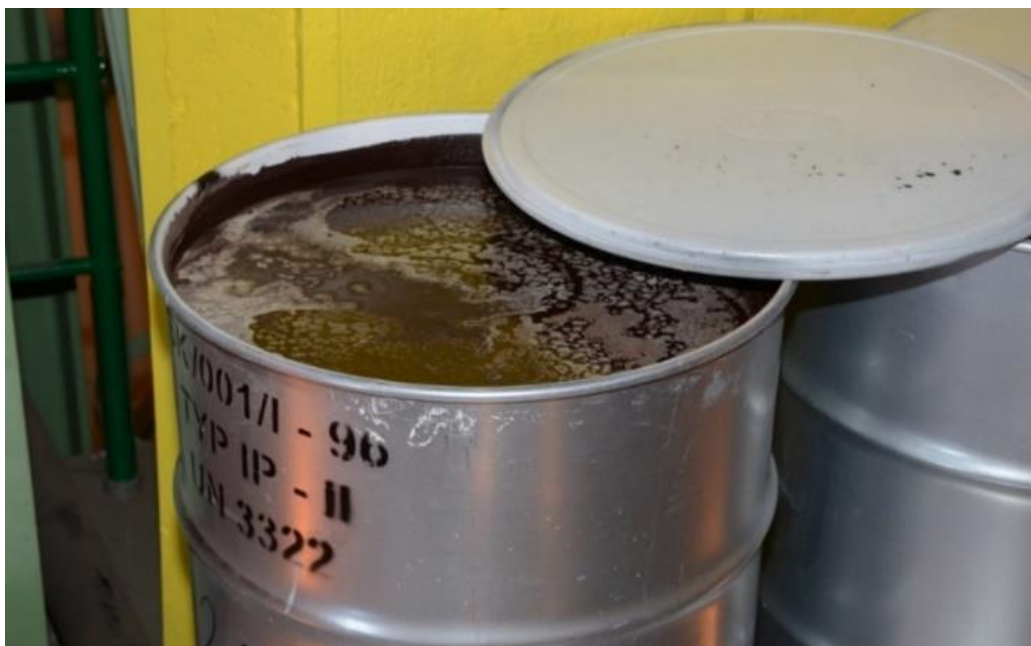
Figure 10. Liquid radioactive waste fixed in an aluminosilicate matrix in a 200 L drum
