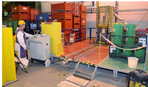
Figure 14. Conveyor belt for transporting drums with liquid RAW for fixation
