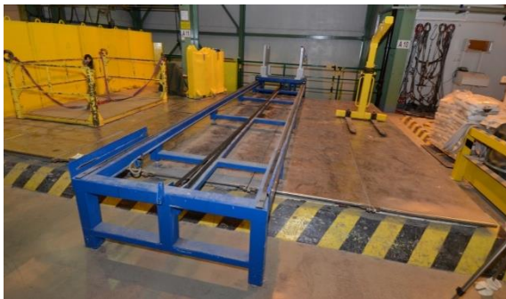
Figure 13. Conveyor belt for transporting drums to the rotating jib crane
