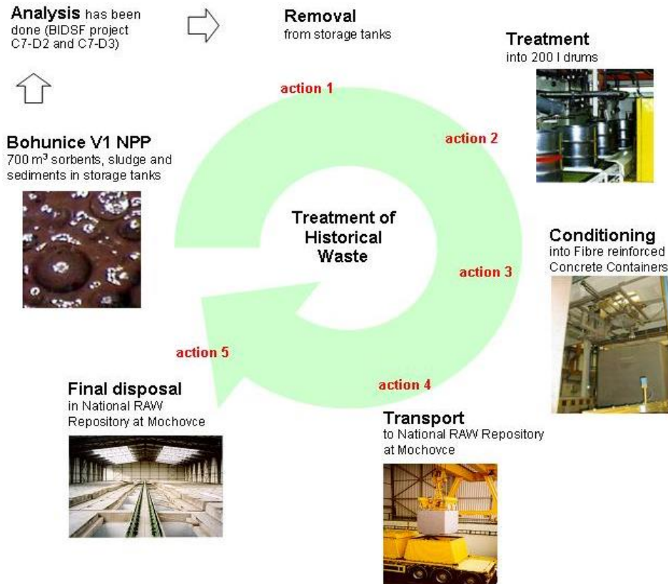
Figure 4. Process of operational liquid radioactive waste management
