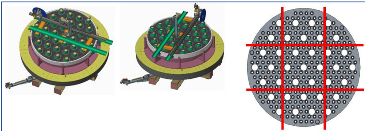
Figure 27. Cutting plan for the top and bottom plates of the bearing shell bottom
