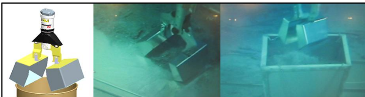
Figure 9. Scooping of chips not captured by exhausting from the bottom of the WCW
