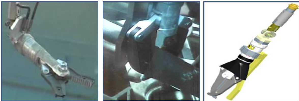
Figure 5. Shearing and clamping equipment (straight, parrot and eagle type)
