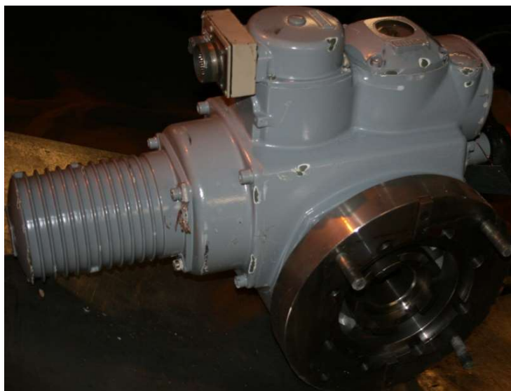
Figure 9. Valve servo actuator prepared for gamma-spectroscopy measurements.
