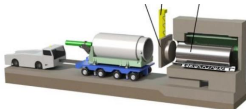
Figure 45. Remove the cask and install the HSM door
