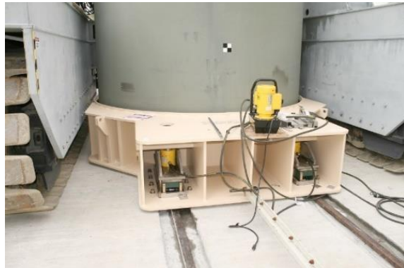
Figure 25. Diagram of a ZPT (left) and ZPT transporting a SC at Ascó NPP (right) [5]
