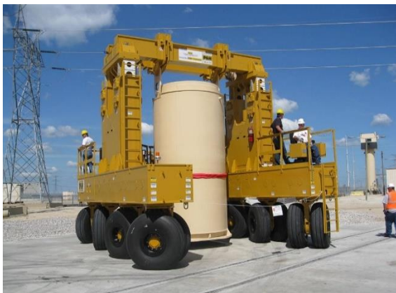
Figure 15. Vehicle for transporting SCs with tyres [8]
