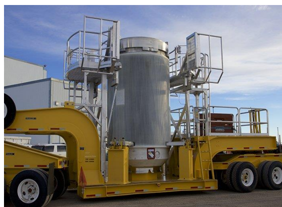
Figure 16. Heavy trailer to move SCs with truck [9]
